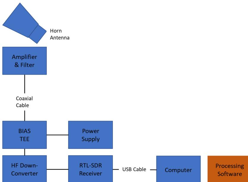
The galactic rotation curve can be calculated by recording a number of frequency spectra measurements with the horn antenna is aimed at a fixed position in the sky and using the Earth's rotation to traverse across the Milky Way galaxy – this method was used by Dr David Morgan<sup>26</sup>.
